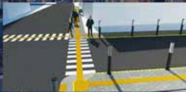
The guiding paths were provided to assist the visually impaired persons to cross the street
