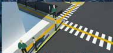
The curb ramps with 1:12 were provided. The additional guiding paths and speed bumps were added.
