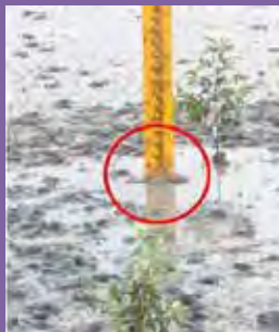
Measure the depth of sludge before applying EM mudballs
